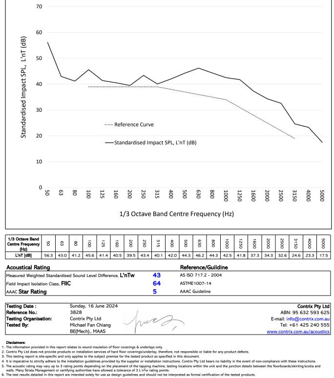
7. The use of any glue or adhesive can negatively impact the acoustic rating. Based on previous testing data, a degradation of up to 5 L'nTw rating points has been recorded. 8. It is highly recommended to engage a qualified acoustic consultant (Contact Contrix Pty Ltd on +61 425 240 555 or other qualified consultants) to conduct in-situ testing (field testing) prior to flooring installation
